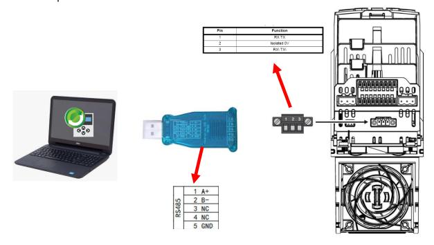
After connecting the interface to the computer, check which USB port the interface has been configured to communicate with Connect.
