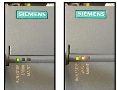
If the PLC is reporting no errors then **S.02.003**, **S.02.004** and **S.05.004** on the drive should also be checked to ensure that the PROFINET network is operating correctly, where they should display that the network is active, has a cyclic data rate greater than 0 and no configuration error has occurred.
