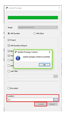
After this procedure, it is possible to verify that a file was created inside the USB stick, this file has a .zip extension and is used in the HMI to download the project that was created.
