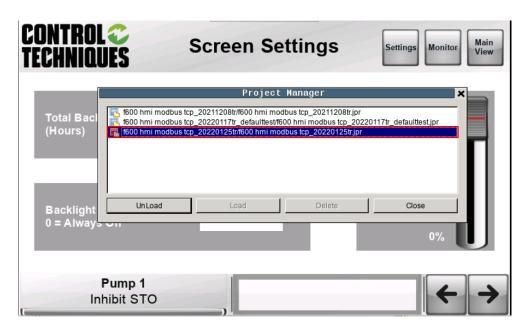
By clicking on "Un Load" as identified below, it is possible to leave the HMI without any software loaded, but they are kept internally in the HMI's memory.
