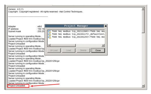
If you want to remove the projects loaded on the HMI or if you don't have enough space to download a new project, delete the files as shown in the image below.
