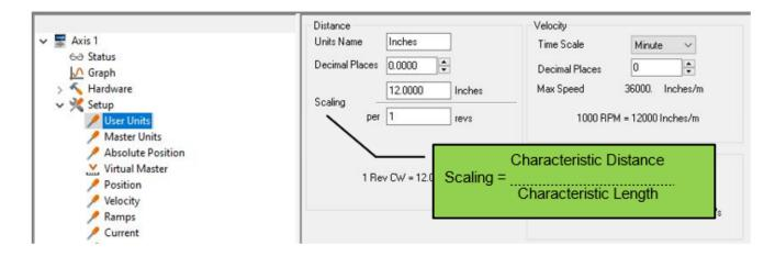
For example, if Dual Loop is enabled and you initiate an index distance of 12 inches and velocity of 24 inches per second, the pinch rolls would drive the material forward 12 inches as measured by the second encoder.
