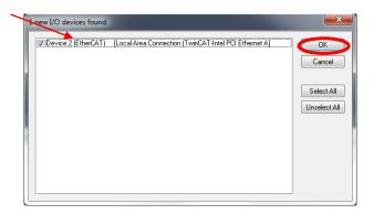
5. Click Yes to scan for EtherCAT™ devices in the network. The correct XML files installed in C:\TwinCAT\lo\EtherCAT will help TwinCAT™ System Manager correctly identify and name each EtherCAT™ node it detects.
