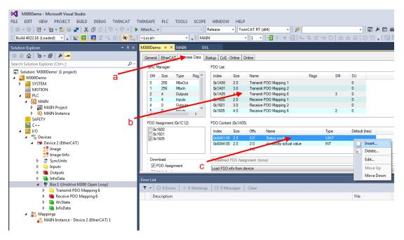
4. In the dictionary, select the drive parameter that will be added to Transmit PDO 6. Use the following to decode the objects in the dicitonary from drive parameters: 0x200A: 65 where A indicates the menu number in hex (10 in decimal) and 65 indicates parameter number in hex (101 in decimal). Select and click OK.
