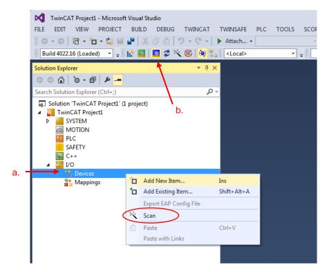
NOTE: If "Scan Devices..." is greyed out in the dropdown list after rightclicking, make sure to go into Config Mode by pressing the icon indicated by (b).
