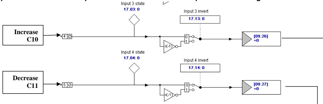
Step 3 is to connect Terminal C10 as the Increase pushbutton by setting #17.23 to 9.26
