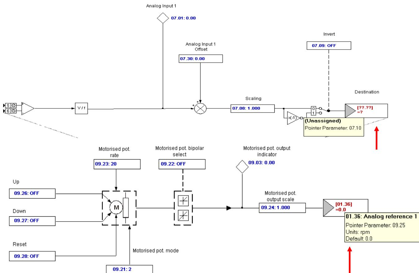
Step 2 is to connect the output of the MOP function to the speed reference register #9.25 = 1.36
