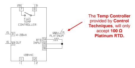
If using a **Two-wire RTD**, then place a jumper between **Terminals 35 & 36** and connect the **RTD** between **Terminals 34 & 35**.
