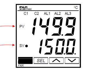
\*If the Setpoint Value needs to be **Degrees Celsius**, then  $\Pi$ – $\Phi$  will have to be changed to  ${}^{\circ}$ C, in the **Second Block**.
