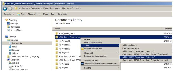
Once the .zip folder has been emailed the recipient can extract the entire folder contents to the default folder location or to a user created project folder. Open Unidrive M Connect software and select File 'Open'. The project that was extracted now shows up in the folder list and can be opened and will include all of the project information including setup information for any SI-Modules if fitted into the drive slots.
