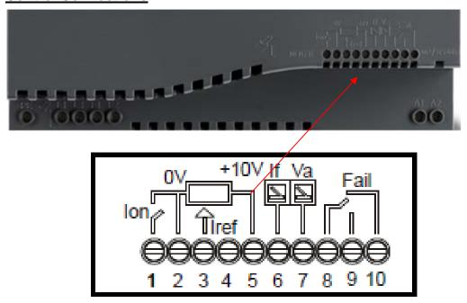
The above diagram shows the basic control connections to the FXMP25.
